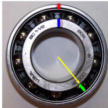
Figure 15. By rotating the inner ring one full rotation the cage has only rotated 40% of a full rotation
