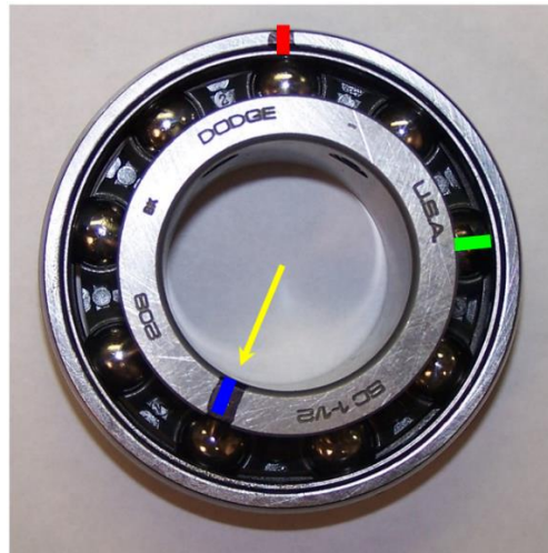
Figure 4. The inner ring mark has just passed the 3 rd ball
