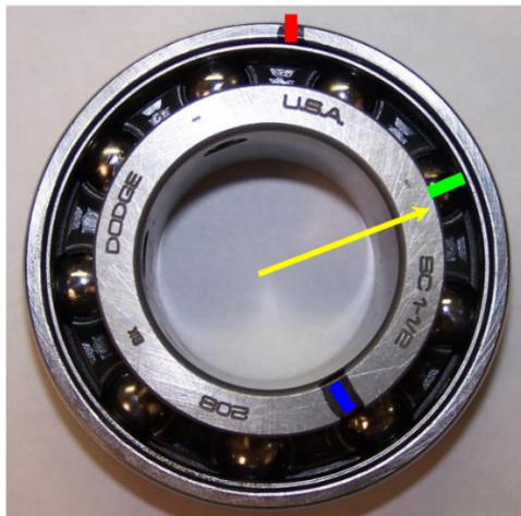
Figure 12. By rotating the inner ring, this illustrates the radial distance the inner ring has rotated before the ball completed one (the first) full rotation (related to the inner and outer ring raceway)
