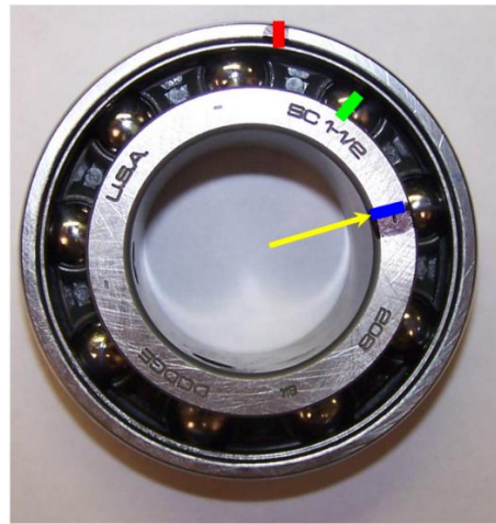
Figure 2. By rotating the inner ring, this illustrates the point at which the blue inner ring match mark passes the first ball
