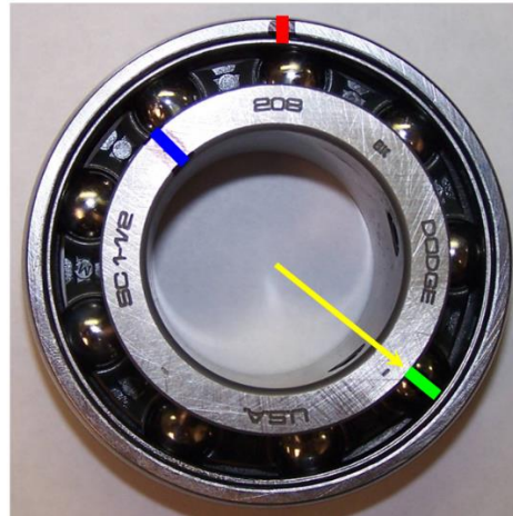
Figure 13. Continuing to rotate the inner ring, this illustrates the radial distance the inner ring has rotated before the ball completed the second full rotation (related to the inner and outer ring raceways).
