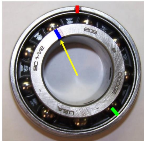
Figure 6. The inner ring mark has just passed the 5 th ball
