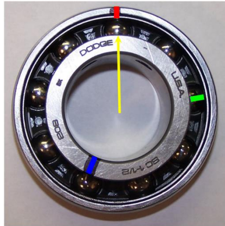
Figure 9. Continuing with the inner ring rotation. This is the point at which the second roller crosses the stationary point on the outer ring
