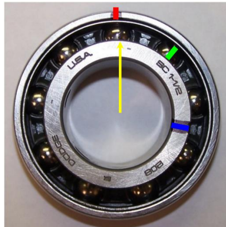
Figure 8. By rotating the inner ring, this illustrates the point at which the first ball has passed a point on the outer ring
