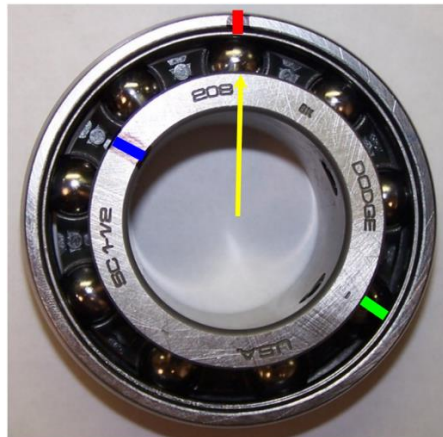
Figure 10. The third roller has now crosses the stationary point on the outer ring
