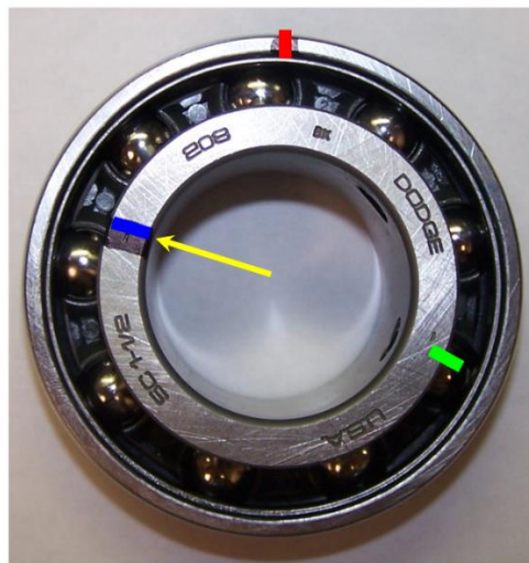
Figure 5. The inner ring mark has just passed the 4 th ball
