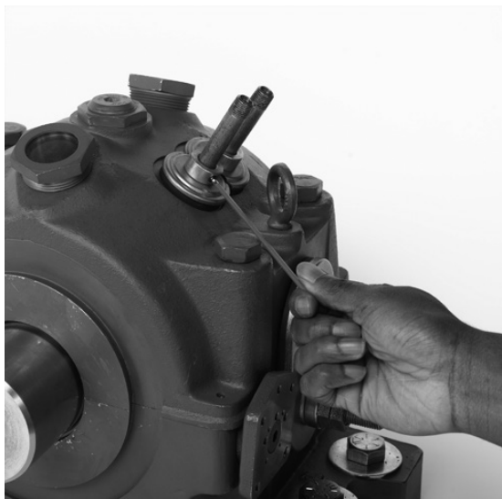
Figure 5 - RTL Circulating Oil Inlets
