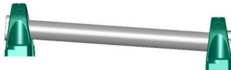
Figure 2. Static Misalignment Side View
