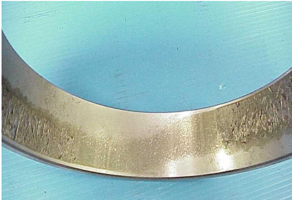
Figure 4. Meandering Wear Pattern
