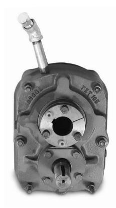
Dodge Torque-Arm speed reducer. The speed reducer shall be either a belt driven or direct coupled enclosed shaft mount type unit with a single or double reduction ratio. The reducer shall mount directly on the driven shaft and utilize an adjustable Torque-Arm that attaches from the gear case to the support structure or foundation.
