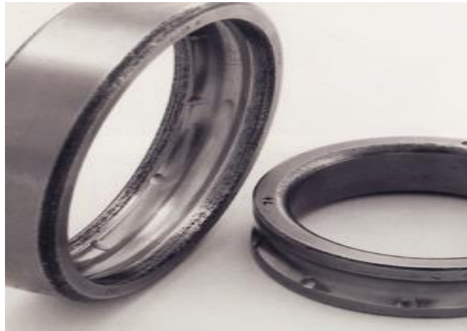
Figure 2. Axial shock load on a ball bearing
