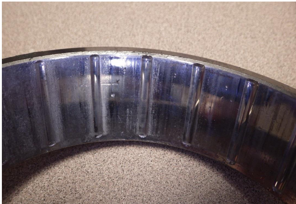
Figure 1. Roller indentations on taper bearing cup
