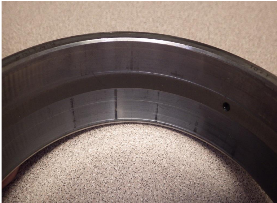
Figure 4. Outer race showing false brinelling
