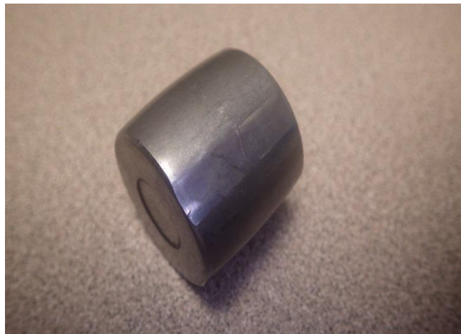
Figure 3. Roller from spherical roller bearing damaged by brinelling
