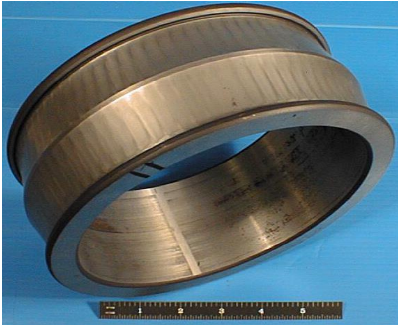
Figure 5: Inner ring showing damage from vibration
