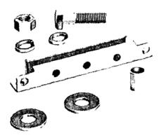
The chain tensioner frame may be mounted on surfaces parallel to or at 90° to the plane of the chain drive. Mounting is accomplished by using two 5/16" dia. bolts, provided by the user. Parallel surface mounting provides a full 4" of adjustment. Installation on a surface 90° to the chain drive, will limit adjustment to 2½" or 1½", depending on which intermediate mounting hole is used.
