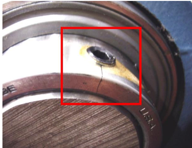
Figure 1. Cracked ball bearing inner ring
