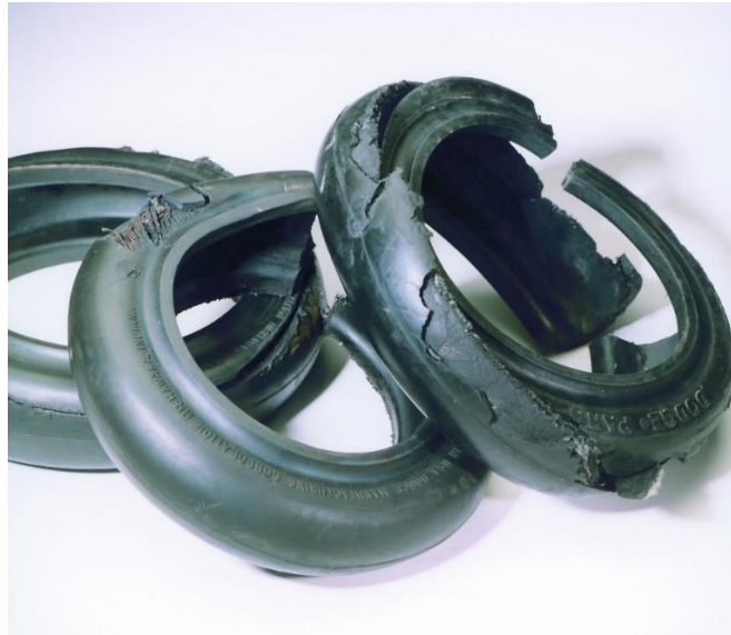
Figure 1. Torsional Overload Failures
