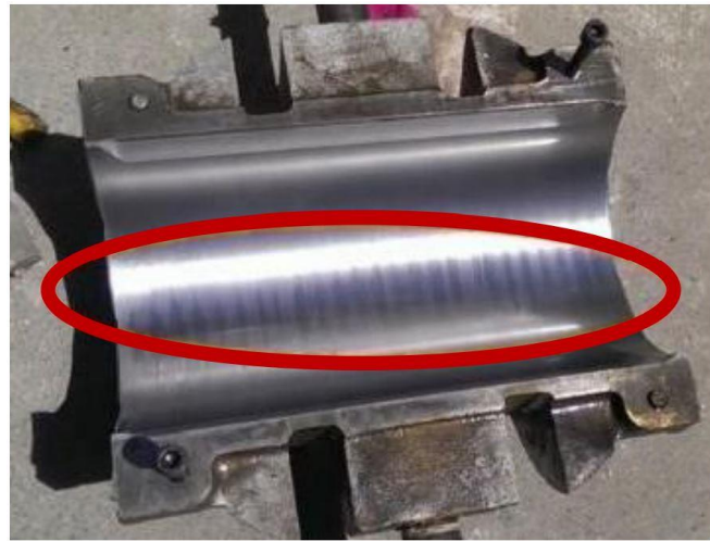
Figure 6. Babbitt-lined bearing conformed to imperfections on the shaft.
