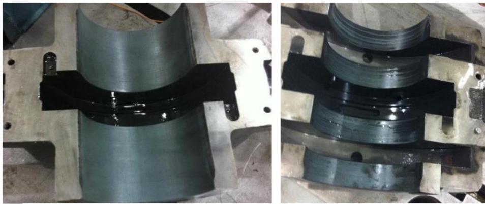
Figure 8. PTFE-based lower half (left) and upper half (right) after approximately 1000 hours of testing
