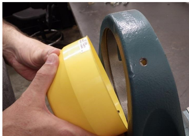
Figure 3. Starting position of the end cover.
