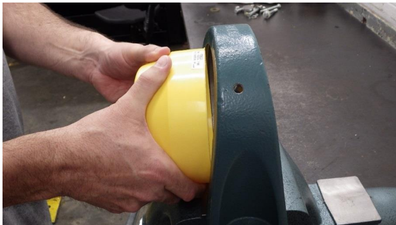
Figure 4. Lip being inserted along one side.
