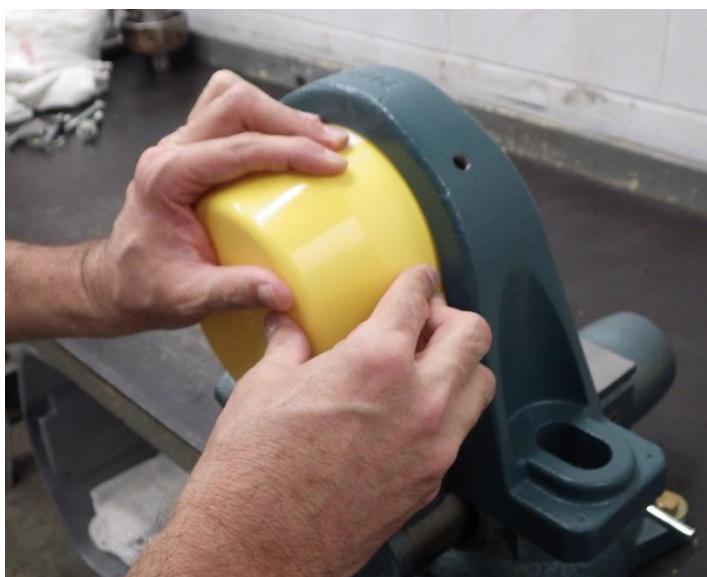
Figure 7. Last portion of raised lip being fitted.
