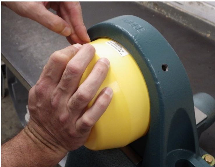
Figure 6. Cap being pressed to allow raised lip to seat.
