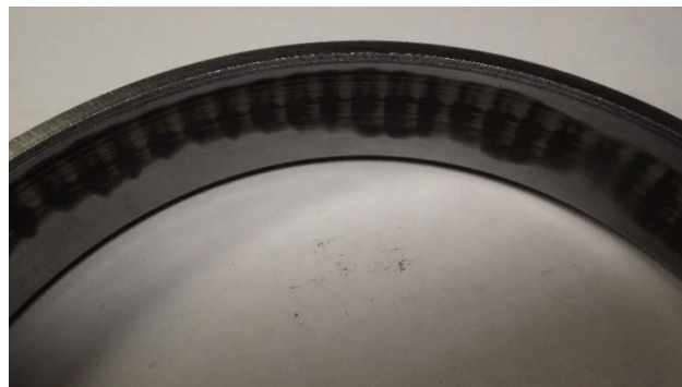
Image 5. Wash board pattern from rolling elements passing through damaged raceways
