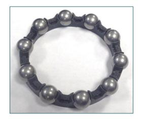
With most standard cages, as shown above, grease is blocked from reaching the back side of the bearing. Also, because there are no pockets to hold it in place, grease has a tendency to be pushed to the other side of the bearing cavity as the rollers churn through it. The graphic below simulates the grease moving to the side of the cavity.
