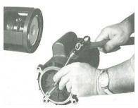
Slide motor shaft into FLEXIDYNE unit. Install and tighten bolts. Locate rubber element so that it is flush with knurled end of C-FLEX module output shaft. Locate clamp flush with end of rubber element and tighten clamp screw snugly.
