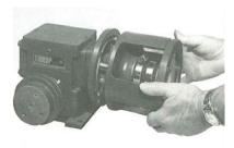
4. Stake the motor shaft key in position, flush with end of motor shaft.
