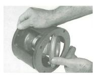
It is recommended that the reducer be firmly attached to its support before installing C-FLEX module and motor. Stake C-FLEX module output shaft key in position and insert module into reducer. Install and tighten bolts to 360 in-lbs.
