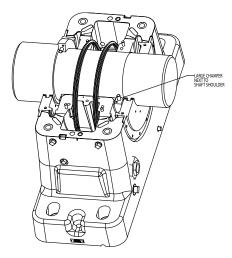
NOTE: Collar halves are match marked; do NOT assemble halves with different marks.
