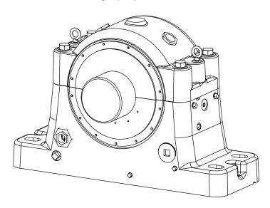
NOTE: Align dowel pin and dowel pin hole in housing halves before lowering cap onto base.
