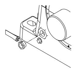
Note: Each housing base has two pre-drilled holes for doweling housing to pedestal.
