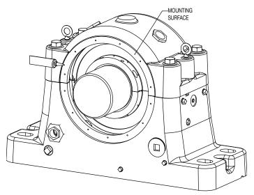
Assemble each seal around shaft and torque clamp screws to value specified in Table 6.
