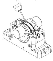
NOTE: 'T' liners have a rotation direction arrow mounted to top of upper liner; arrow MUST point in same direction as rotation of top of shaft. If not, liner must be removed, reversed and reinstalled so arrow points in proper direction.
