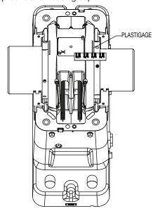
Compare the width of the deformed Plastigage with the inch scale on its wrapper. This indicates the clearance between housing and liner.
