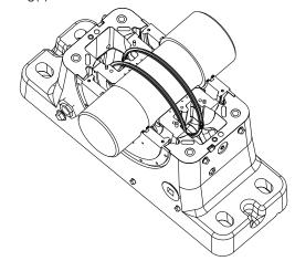
Install and tighten four screws in each oil ring using a low strength thread locker.
