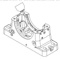
Apply oil to the spherical seats of the housing base and to the spherical seats of the lower liner half. The lower liner half is identified by its continuous babbitted bore surface; the upper liner half has one or two oil ring slot(s) in the center of the babbitted bore.
