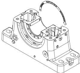
NOTE: 'T' liner must be installed in direct relationship with shaft rotation.
