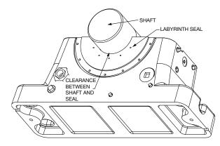
Alignment of pillow block should be accurate since the self-aligning feature of the bearing is to compensate for normal shaft deflection.
