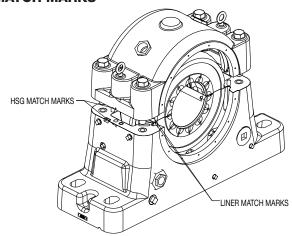
All SLEEVOIL housing and liner halves have match marks permanently stamped above and below the joint. Use these match marks to ensure that parts stay paired and critical machined areas of an assembly are accurately maintained.
