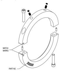
Place one half of collar on shaft with large chamfer next to shaft shoulder. Rotate collar half around shaft and place other half in position.
