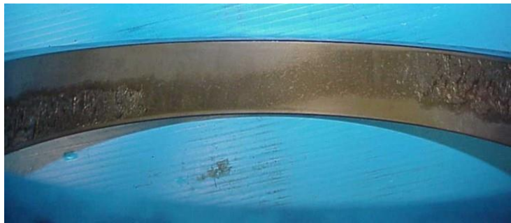
Figure 4. Close-up of cup/cone assembly (left) and wear pattern on bearing cone (right)
