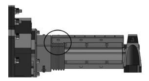
5. Pinch the flanges of both halves tight to ensure the ribs of the extension are fully engaged with the ribs of the adapter.
