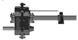
Once this distance is known, use the reference measurements on the OD of the extension to cut it to the appropriate length. For longer distances, it may be beneficial to have the extension reach over top of the connecting piece of equipment for extra support.
