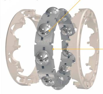
Unlike standard designs, the Maxlife cage holds a large volume of grease which ensures constant contact with the rolling elements
