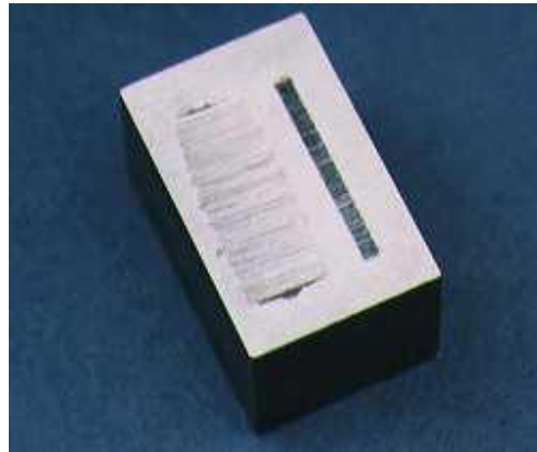
Figure 2. Sample of Scarring on Test Block
