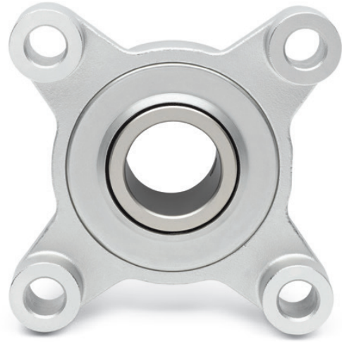
Figure 3 - Four Bolt Flange Standoff Bearing with Backside Seal Installed
