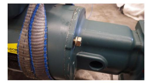
Once the motor tenon has been separated from the reducer, support the motor fan end and keep constant axial pressure on the fan shroud towards the reducer. This pressure is required to keep the three piece coupling halves from disengaging and must be maintained throughout the motor rotation procedure. Remove the two remaining motor mounting capscrews.
