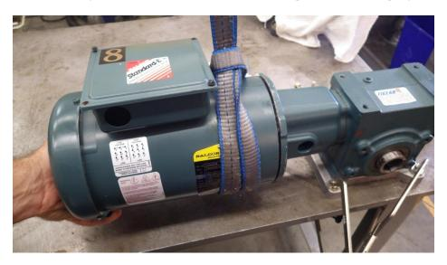
Slowly rotate the motor to the desired conduit box position. The lifting strap / straps may have
