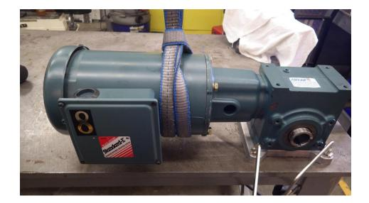
• Look into the coupling access hole and verify the three piece coupling is properly engage.
