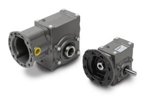
E-Z Kleen reducers are washdown ready and corrosion resistant. The totally enclosed ventless sealing system contains a factory-filled food grade synthetic lubricant that eliminates the need for routine oil changes.
